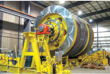
Hepburn 192-in. Modified Blair Service Hoist during factory assembly. When installed, the hoist will be used to lift the world's largest personnel cage.
