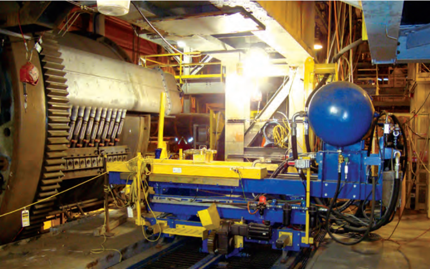
The Gaspé Puncher Automatic clears the Tuyère pipe openings in the converter vessel of Cu & Ni smelters thereby making the smelting process more efficient.
