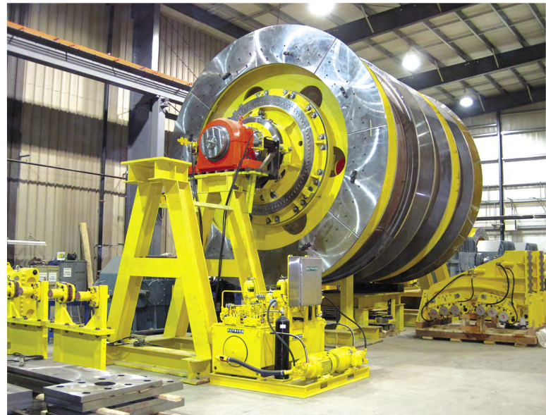
Hepburn 192-in. Modified Blair Service Hoist during factory assembly. When installed, the hoist will be used to lift the world's largest personnel cage.
