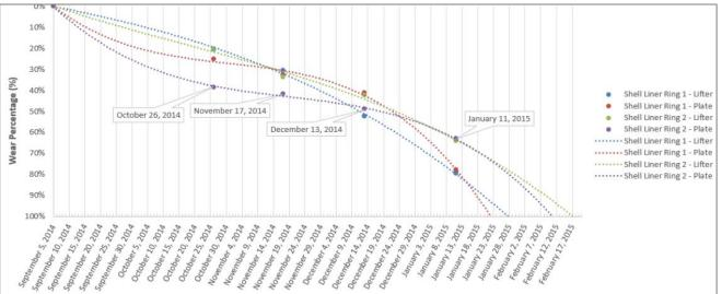
It is recommended that the mills each be scanned five times throughput their respective liner lives, or once per quarter, whichever is sooner. Utilizing algorithms derived from present and historical data, the liner wear forecast dates are predicted with high accuracy. This allows the client to reline the mill exactly when needed, saving money on mill downtime, reducing overall milling costs, and using the liners to their full potential.
