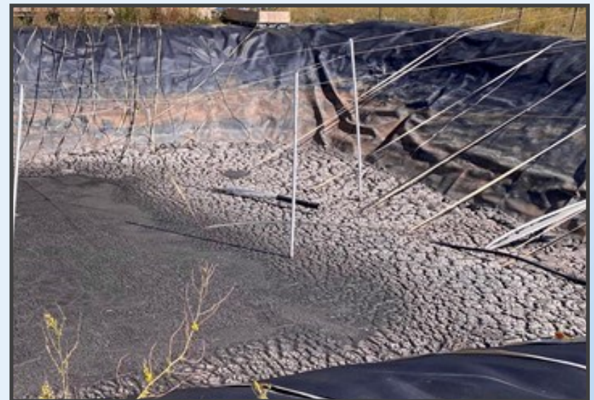
Consolidated tailings after 19 months of treatment
