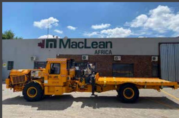
The 2016 introduction of the MacLean EV Series™ of zero emissions/DPM, low maintenance, low heat, low noise, data-rich, high performance mining vehicles was a product development milestone for the company. Since then, we have gone on to manufacture and commission over 40 battery electric mining vehicles (BEVs) at underground mines globally, with over 100,000+ operating hours to date.
