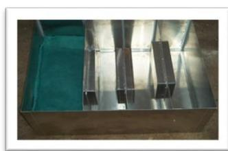
This three stage separator ensures that a busy automotive car dealership meets local bylaws. Oil and sludge largely settle in the first two stages.
