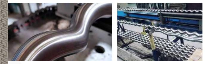
Type of grinding machines: Several set-ups are possible to reach the required finish. Stationary belt grinders provide a consistent finish where manual belt grinders allow the finishing of more difficult to reach areas.
