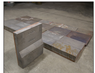
APRON FEEDER LINERS - BIG FOOT, DOMITE BOLTS, GRAV LOCK, DOMITE CERAMIC (IN BETA TESTING)
