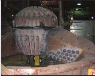
SPIDER ARM / RIM PROTECTION - DOMITE OCTAGON, CHOCKY BARS, BUTTONS, BLOCKS, GRAV LOCK
