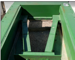
LOAD OUT V / DISCHARGE LIP - MINI LOAF, TRANSFER POINT LINER, CAST BLOCKS
