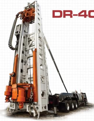
Foremost's first fully electric drill features a remote console for operator safety. The DR-40SHD features a brand new 40" lower drive with increased capacity and improved chucking system. Utilizing the flexibility to drill anywhere from vertical to horizontal angles, the DR-40SHD can be used in a wide variety of applications including de-salination projects and deep hole water wells.
