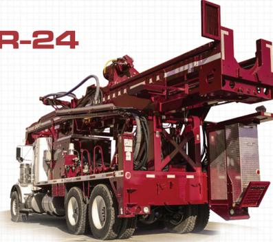
The DR-24 will set casing up to 24" (610 mm) in diameter. This model is commonly used for domestic and municipal wells, and construction applications such as foundation piling projects and holes for hydraulic elevator jacks. The DR-24 is available in PTO or deck engine configurations and can be mounted on a truck, trailer or self-propelled tracked carrier. Available in a stock tandem (pictured above) or tridem configuration.
