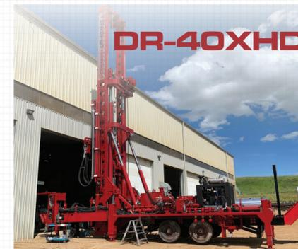
Building on the technology behind the DR-24XHD, the DR-40XHD features the DR-40 lower drive with increased pullback capability. The DR-40XHD can also be configured with an angle package, with the ability to drill on an angle from 0-45 degrees. The DR-40XHD excels in deep hole large diameter waterwell and construction applications.
