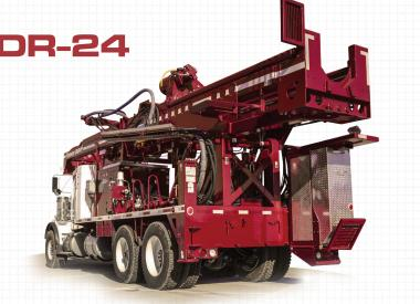
The DR-24 will set casing up to 24" (610 mm) in diameter. This model is commonly used for domestic and municipal wells, and construction applications such as foundation piling projects and holes for hydraulic elevator jacks. The DR-24 is available in PTO or deck engine configurations and can be mounted on a truck, trailer or self-propelled tracked carrier. Available in a stock tandem (pictured above) or tridem configuration.
