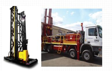
For some applications, the Foremost DR Drill may not be suitable on a traditional chassis. All the versatility of the Foremost Dual Rotary Drill can be mounted on virtually any non-standard North American Chassis (pictured top-right), or installed and mounted onto crane leads (pictured top-left).
