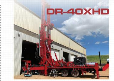
Building on the technology behind the DR-24XHD, the DR-40XHD features the DR-40 lower drive with increased pullback capability. The DR-40XHD can also be configured with an angle package, with the ability to drill on an angle from 0-45 degrees. The DR-40XHD excels in deep hole large diameter waterwell and construction applications.
