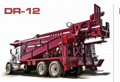
The DR-12 is a light, yet powerful PTO rig popular among domestic water well contractors drilling in moderate to severe overburden. It will handle casing up to 12" (305 mm) in diameter, and has been field tested to depths beyond 550 ft (168 m) for a typical 6" (152 mm) cased well. The DR-12 is available with an optional pipe tub, single pipe loader arm and telescopic casing jib. The configuration accommodates diverse site conditions.
