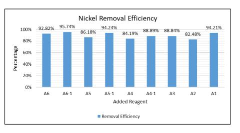
Results of treating site sample with acidic water (pH=1.94) containing different dosages of PMAP reagent. The pH of treated water won't be higher than 9 either at optimum dosage (A6-1) or at 2.5-time excessive reagent consumption (A1).
