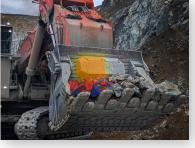
ShovelSense<sup>®</sup> real-time ore characterization in each bucket enables ore sorting at extraction face
