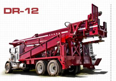
The DR-12 is a light, yet powerful PTO rig popular among domestic water well contractors drilling in moderate to severe overburden. It will handle casing up to 12" (305 mm) in diameter, and has been field tested to depths beyond 550 ft (168 m) for a typical 6" (152 mm) cased well. The DR-12 is available with an optional pipe tub, single pipe loader arm and telescopic casing jib. The configuration accommodates diverse site conditions.
