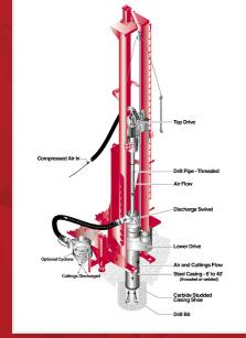
ower rotary casing drive is used as a breakout and spinner wrench for drill pipe joints, drill bits, and threaded casing
