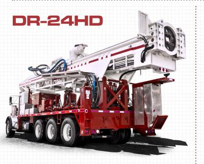
The DR-24HD ('heavy-duty') features a heavy-duty gear-driven lower drive, which generates two and a half times the torque of the standard DR-24. The DR-24HD is also configured with a heavy-duty mast to withstand the additional torque and larger hoist cylinders for increased pullback capabilities. The DR-24HD is most commonly used in deep, large diameter applications such as municipal/industrial wells and mine de-watering.
