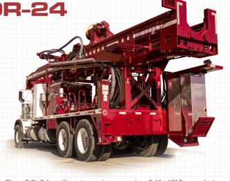
The DR-24 will set casing up to 24" (610 mm) in diameter. This model is commonly used for domestic and municipal wells, and construction applications such as foundation piling projects and holes for hydraulic elevator jacks. The DR-24 is available in PTO or deck engine configurations and can be mounted on a truck, trailer or self-propelled tracked carrier. Available in a stock tandem (pictured above) or tridem configuration.
