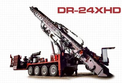
The DR-24XHD features the DR-24HD lower drive with increased top drive torque and pullback capability. The DR-24XHD is also configured with an angle package, with the ability to drill on an angle from 0-45 degrees. The DR-24XHD excels in deep hole waterwell and mine dewatering applications.
