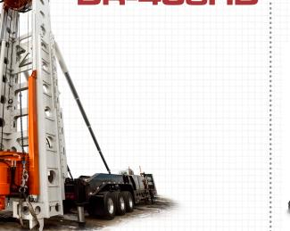
Foremost's first fully electric drill features a remote console for operator safety. The DR-40SHD features a brand new 40" lower drive with increased capacity and improved chucking system. Utilizing the flexibility to drill anywhere from vertical to horizontal angles, the DR-40SHD can used in a wide variety of applications including de-salination projects and deep hole water
