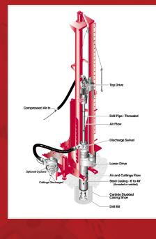
Lower rotary casing drive is used as a breakout and spinner wrench for drill pipe joints, drill bits, and threaded casing.
