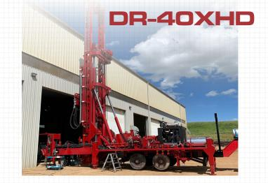
Building on the technology behind the DR-24XHD, the DR-40XHD features the DR-40 lower drive with increased pullback capability. The DR-40XHD can also be configured with an angle package, with the ability to drill on an angle from 0-45 degrees. The DR-40XHD excels in deep hole large diameter waterwell and
